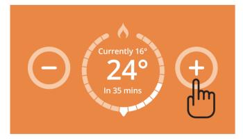
To INCREASE the current temperature, repeatedly press the 🛨 button on the Switchee thermostat until your desired temperature is displayed centrally.
