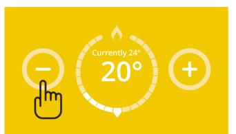
To DECREASE the current temperature, repeatedly press the **button** on the Switchee thermostat until your desired temperature is displayed centrally.
