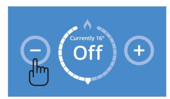
Repeatedly press the **button** on the **Switchee thermostat** until the **desired temperature** displayed centrally is lower than the **current temperature**.
