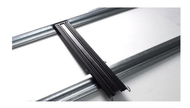
The metal batten is installed like a traditional timber batten. These are installed at 307mm apart
